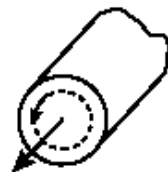
Magnetic field inside conductor
